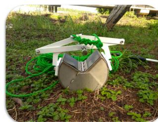
Fig.1: Sediment Grab Sampler
